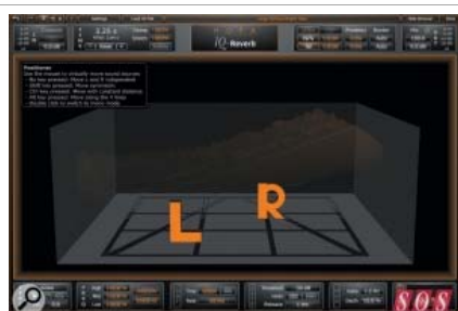
The positioner allows you to place your sources within the virtual space created by IQ Reverb. It works surprisingly well.
